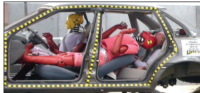
Seat back collapse of a 1992 Dodge Caravan (upper left) and a 2000 Dodge Caravan (upper right). Crash test dummy experiencing a seat back collapse and a head to head collision with a rear seat child occupant (below).
